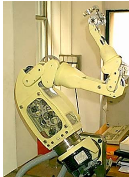
Dexter 8R arm (cables and pulleys)
