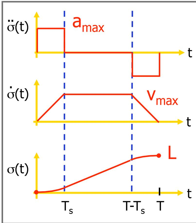
$$\sigma(t) = \begin{cases} a_{\max} t^2/2 & t \in [0, T_s] \\ v_{\max} t - \frac{v_{\max}^2}{2a_{\max}} & t \in [T_s, T-T_s] \\ -a_{\max} (t-T)^2/2 + v_{\max} T - \frac{v_{\max}^2}{a_{\max}} & t \in [T-T_s, T] \end{cases}$$
