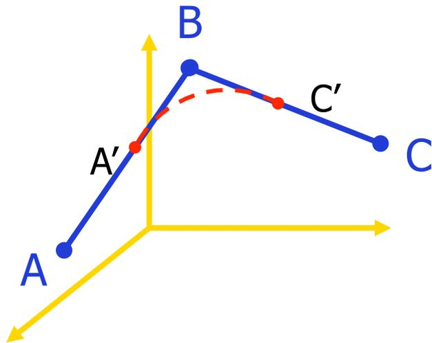
$$\ddot{p}(t) = 1/\Delta T (v_2 K_{BC} - v_1 K_{AB})$$
