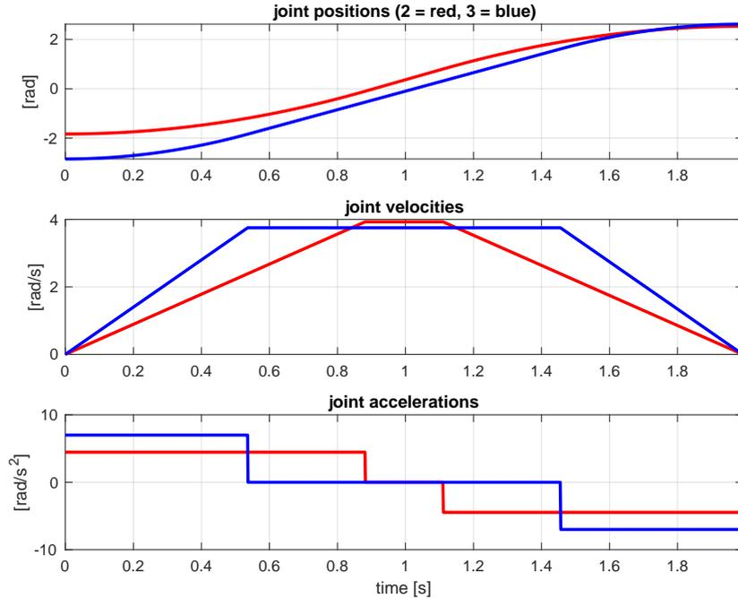
Figure 3: The coordinated minimum-time trajectory for the two joints 2 and 3.
