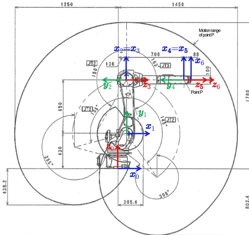
Figure 2: A possible assignment of DH frames for the Kawasaki RS010N robot.
