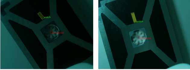
Fig. 3: Result of the inference made by the YOLO model in challenging lighting conditions: dark assumed in Lunar environment. From the patch detection we retrieve the panel orientation, while the connector detection provides the desired position for the end-effector.
