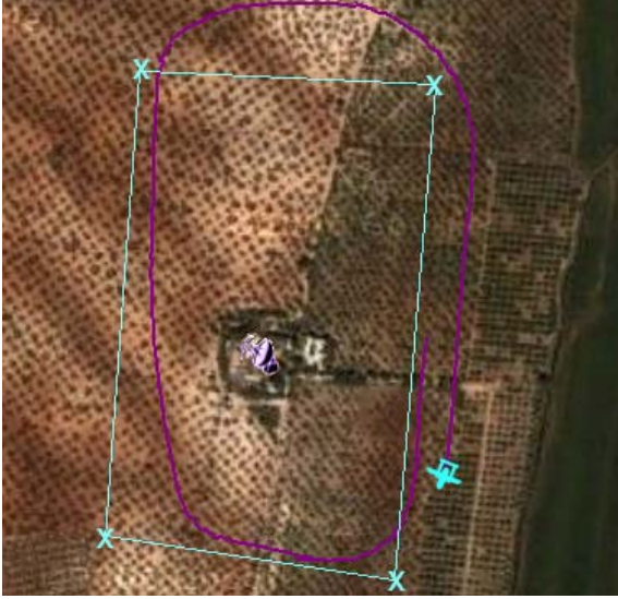
Fig. 2. Tracking of the desired trajectory (blue line) and the real trajectory (violet line) under wind effects
