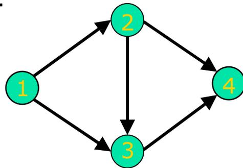
$$M = \begin{array}{c} \begin{array}{ccccc} & 12 & 13 & 23 & 24 & 34 \end{array} \\ \begin{array}{c} 1 \\ 2 \\ 3 \\ 4 \end{array} \begin{array}{|c|c|c|c|c|} \hline -1 & -1 & 0 & 0 & 0 \\ \hline 1 & 0 & -1 & -1 & 0 \\ \hline 0 & 1 & 1 & 0 & -1 \\ \hline 0 & 0 & 0 & 1 & 1 \\ \hline \end{array} \end{array}$$
