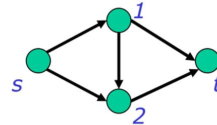
$$\begin{aligned} -\mathbf{x}_{s1} - \mathbf{x}_{s2} &= -1 \\ \mathbf{x}_{1t} + \mathbf{x}_{2t} &= 1 \\ \mathbf{x}_{s1} - \mathbf{x}_{12} - \mathbf{x}_{1t} &= 0 \\ \mathbf{x}_{s2} + \mathbf{x}_{12} - \mathbf{x}_{2t} &= 0 \end{aligned}$$
