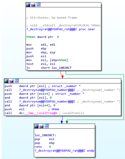
Fig. 4. The instruction at address 10020cf in calc.exe is a join point in the control flow graph of its enclosing function: it can be reached either by a conditional jump from the entry basic block of its function or as a fall-through for the call to the LocalFree API function.
