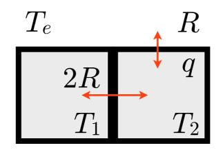
C room thermal capacity R room thermal resistance 2R room thermal resistance between rooms q heat flow source
