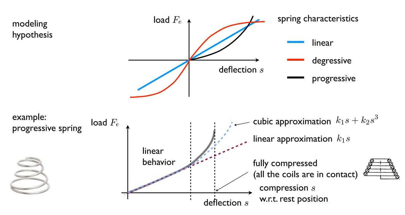
the (linear) approximation of the spring characteristic is part of the modeling phase similarly for the friction force
