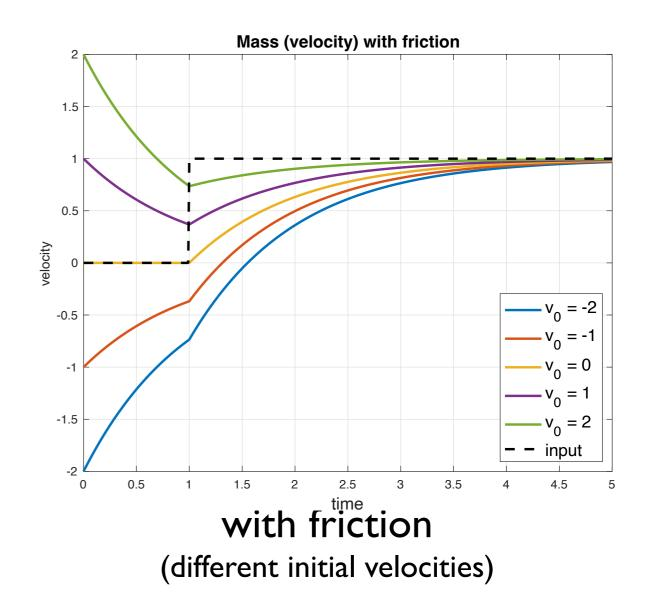
velocity when a constant 1 N force from t = 1 sec is applied
