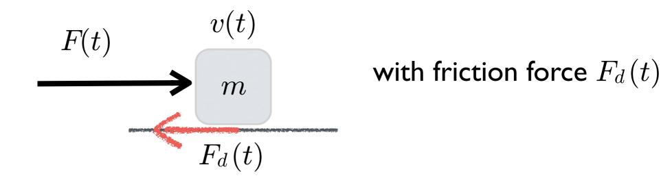
we add a viscous friction force  $F_d(t)$ , acting on the mass, which can be considered proportional to the velocity and acts in the opposite direction
