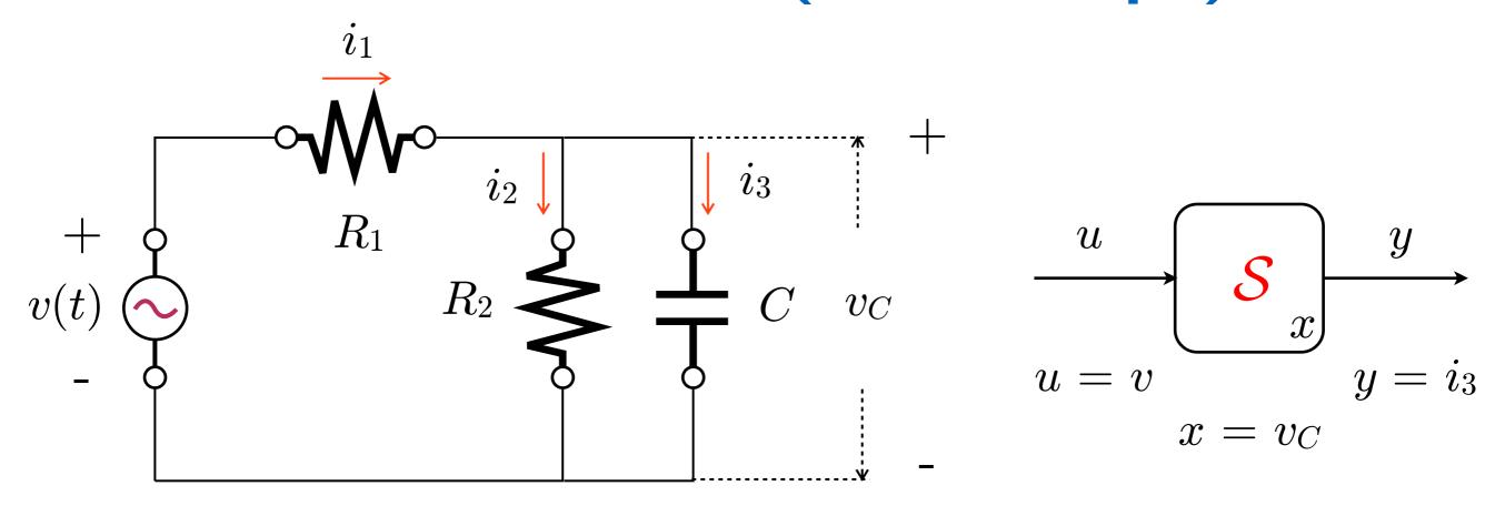
$$\dot{x} = -\frac{1}{C} \left( \frac{1}{R_1} + \frac{1}{R_2} \right) x + \frac{1}{R_1 C} u$$
