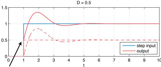
at time t=1, the input switches from 0 to 1 and instantaneously the output switches from 0 to  $D_2 u(1) = D_2$
