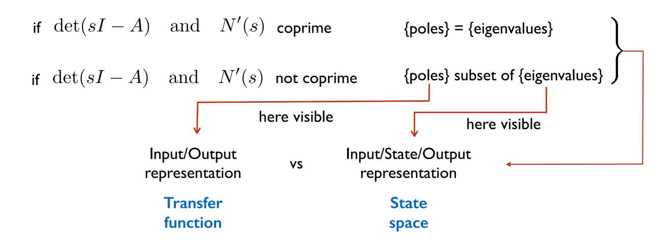
we need to understand when & why this happens (so to understand when we can consider the transfer function equivalent to a state space representation)
