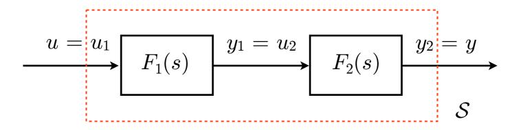
If, in the series of two systems  $F_1(s) = N_1(s)/D_1(s)$  and  $F_2(s) = N_2(s)/D_2(s)$  we have cancellations of common factors between  $N_1(s)$  and  $D_2(s)$  (zero/pole cancellation) or between  $D_1(s)$  and  $N_2(s)$  (pole/zero cancellation), we generate hidden dynamics which can either be uncontrollable or unobservable
