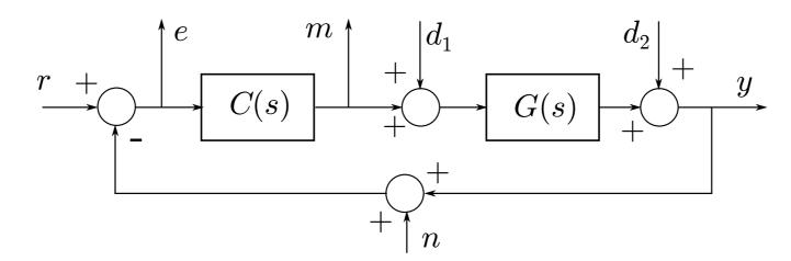
the superposition principle allows us to compute separately each contribution to the chosen output
