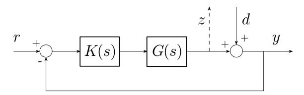
imagine that, for the feedback system shown in figure, we are interested in analyzing the effect of the input d (disturbance) on the output of the system G(s), that is on z
