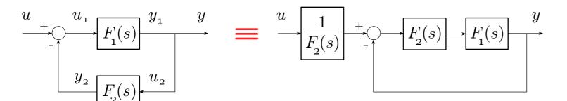
equivalence can be easily shown comparing the signals (their Laplace transforms)
