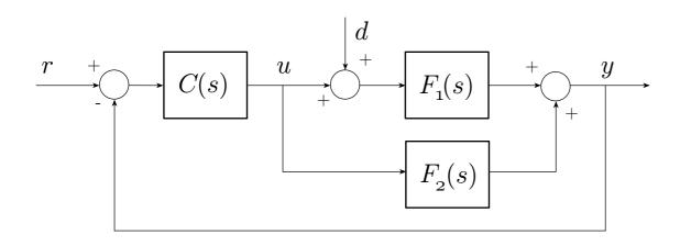
find the two transfer functions  $W_{dy}(s)$  and  $W_{ry}(s)$
