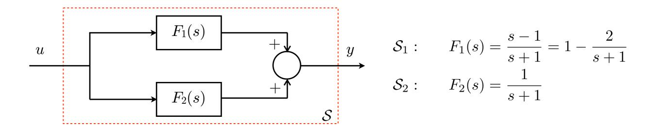
$$F(s) = F_1(s) + F_2(s) = \frac{s-1}{s+1} + \frac{1}{s+1} = \frac{s}{s+1} = 1 - \frac{1}{s+1} \quad \bullet \quad \quad 1 \text{ pole but 2 eigenvalues}$$
