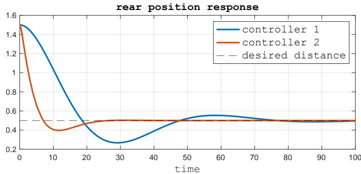
Figure 10: Control scheme comparison - rear position starting from a distance of 1.5 m and p^{\text{sec}} = 0.5 m.
