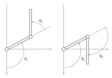
Among the infinite equilibrium configurations, four are unforced (i.e.,  $u_e = 0$ ). They are clearly the up-up configuration  $q_{uu} = (\pi, 0)$ , the up-down configuration  $q_{ud} = (\pi, \pi)$ , the down-down configuration  $q_{dd} = (0, 0)$  and the down-up configuration  $q_{du} = (0, \pi)$ .
