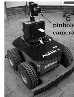
Fig. 16. Mobile robot Pioneer 3X-DE used for the experiments, equipped with the LU175C pinhole camera by Lumenera.
