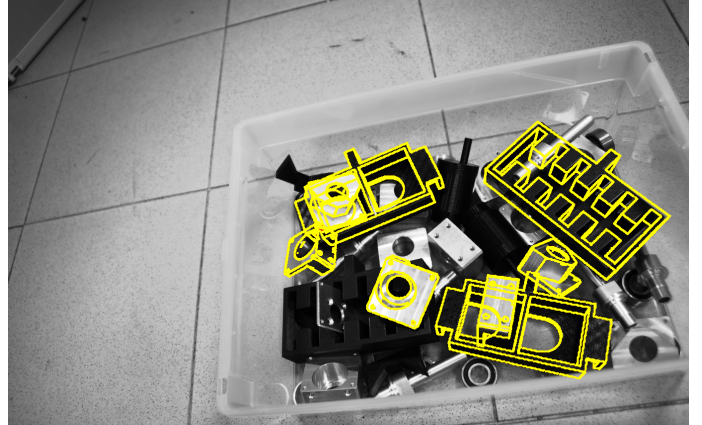
Figure 2: Some object detection and localization results obtained with the proposed active perception strategy (in this examples we are detecting three types of objects).
